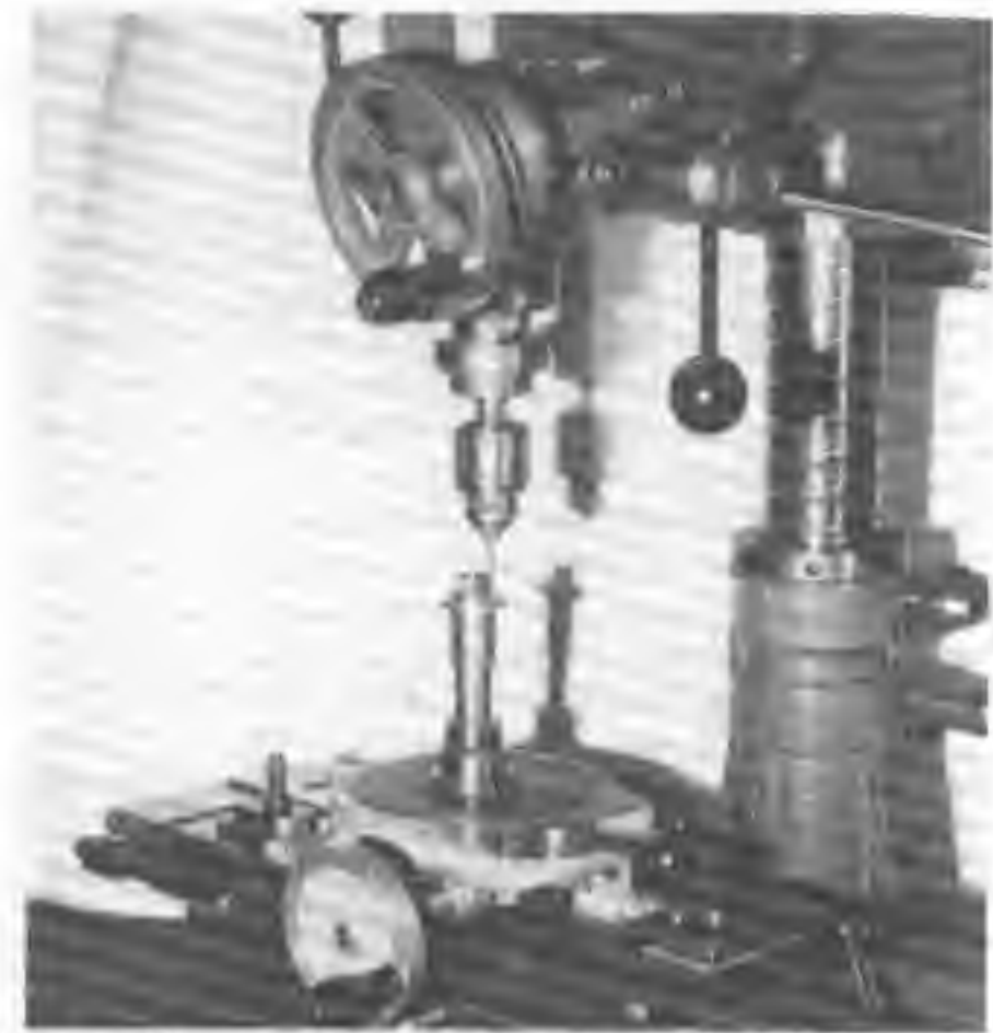
Fig. 109 Drilling the holes in a cutter blank. The indexing is obtained by means of a rotary table.
